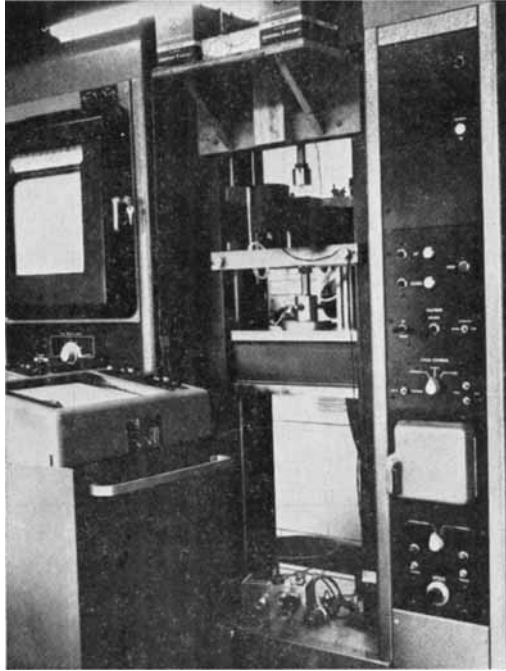
Fig. 21. Assembly of apparatus for controlled strain and strain rate tests.
